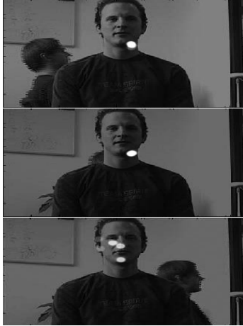
Fig. 2. Three frames from a movie showing one speaker and one moving person. The identified pixels are overlaid as white points in the frames, where intensity is proportional to the corresponding weight \beta_j . Nonnegative CCA clearly identified the audio source in the presence of uncorrelated movements.
