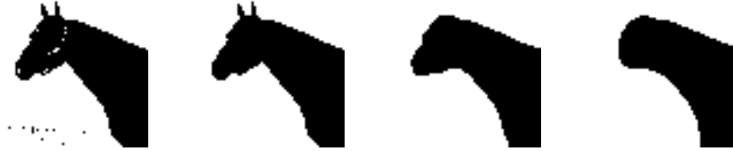
Fig. 3. From left to right: segmentation without total variational smoothing, with \lambda = 0.5 (visually closest to ground truth), with \lambda = 5 and with \lambda = 10
